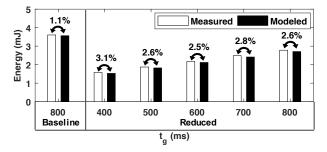
Fig. 6. Comparison of the energy consumed per gesture with the measured data. The number above the bars shows the mean percentage error.
