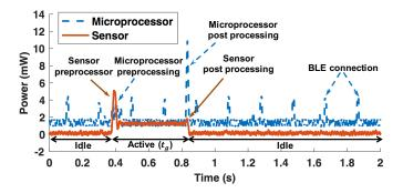
Fig. 5. Power consumption during a gesture recognition when  $t_g=400$  ms.
