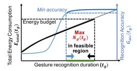
Fig. 3. Energy budget and minimum accuracy requirements constrain the gesture recognition duration  $t_g$  from above and below, respectively. Hence, we maximize the number of recognized gestures within the feasible region.
